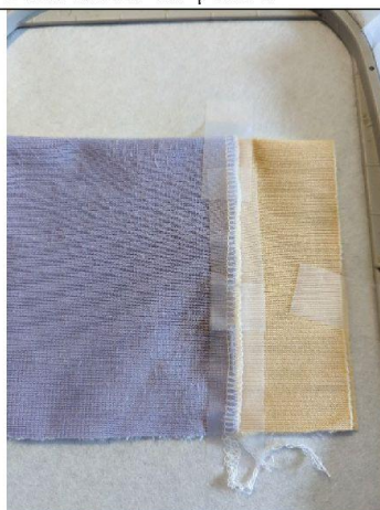
Here I put adhesive tape so that my embroiderer's foot does not get caught in the seam
