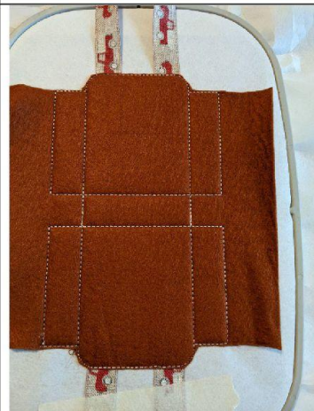
Cut the excess fabric on the top and bottom of the bag only on the back of the frame
