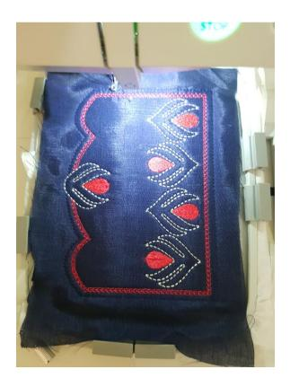
4. Next lay the fabric for the pocket following the size guide for different size of bags. Making sure it is aligned with the placement line, tape it in place and sew the 6<sup>th</sup> color which will tack down the pocket.
