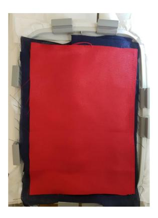
6. Unhoop, Tearaway all the excess stabilizer and trim the bag carefully leaving 1 cm seam all around, leave a little extra at the opening.
