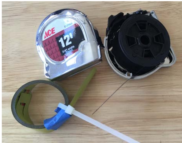
Figure 2. Get a tape measure you can take apart. The removed tape is secured with a tie wrap and some painter's tape.
