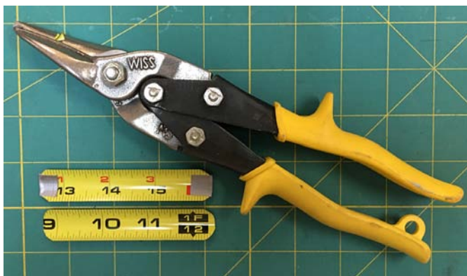
Figure 26. Cut tape measure segments to size, round off ends, and cover with tape.
