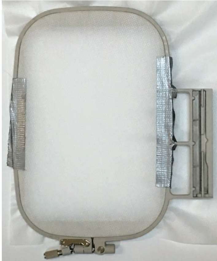
Figure 7. I like to use duct tape to prevent slippage.
