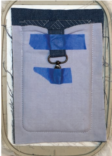
Figure 19. Tape down loop and hardware to keep it out of the final seam.
