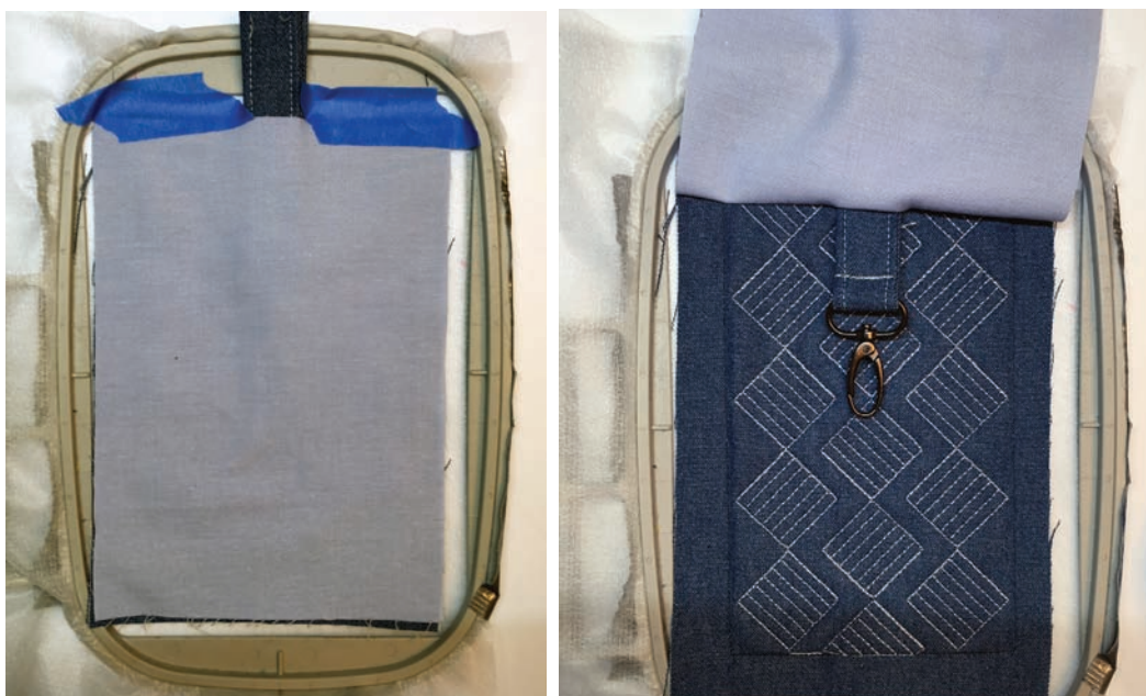
Figure 15. Lining is placed right side down and will be stitched just across the top.
