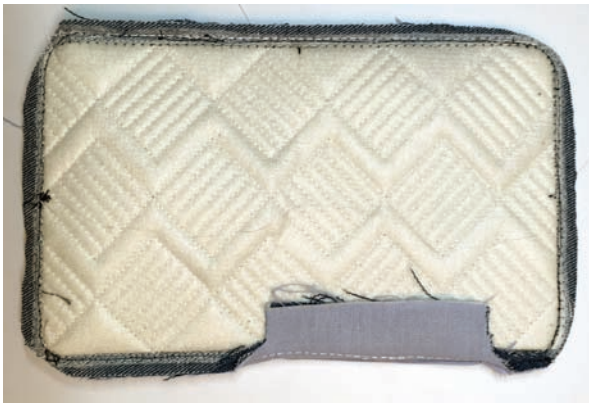
Figure 20. Seam extensions at the turn opening have been pressed back. The thicker side has been fused down with fusible tape to make a neater edge.
