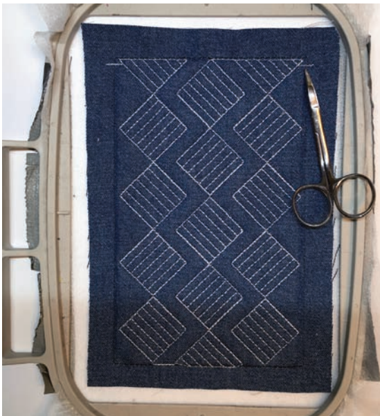
Figure 17. Front panel is stitched and the placement guides indicate where to align the upper edge of the back panel. The back panel must be at or below these guides to avoid stitching the back closed.
