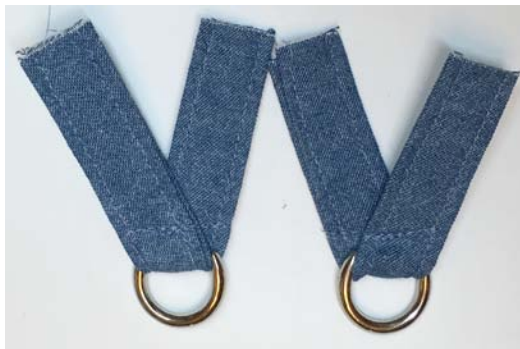
Figure 7. Straps made in this manner can be very thick and when folded over for loops will be 8 layers of fabric. Consider distributing the thickness by shaping pieces that will be sewn into the seam in the hoop into "v."
