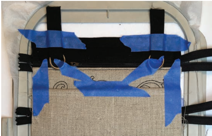
Figure 36. Apply tape over areas that could trip the foot to create a “ramp” the presser foot can glide over.
