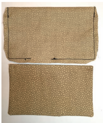
Figure 9. Fold rectangle in half, right sides together, stitch leaving an opening for turning. Turn right side out, press, and top stitch along top edge before stitching to your bag lining.
