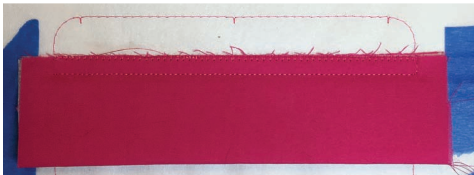
Figure 25. Raw edge is zigzagged to edge of zipper tape and then a straight seam attaches the panel to the zipper. This seam will be used as a fold line and the later top stitching will provide additional security.
