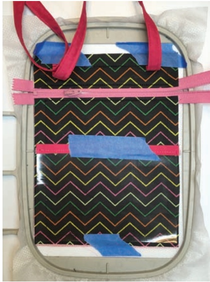
Figure 23. Secure the pocket, positioning it as desired making sure the bottom and sides extend over the tack down stitching.
