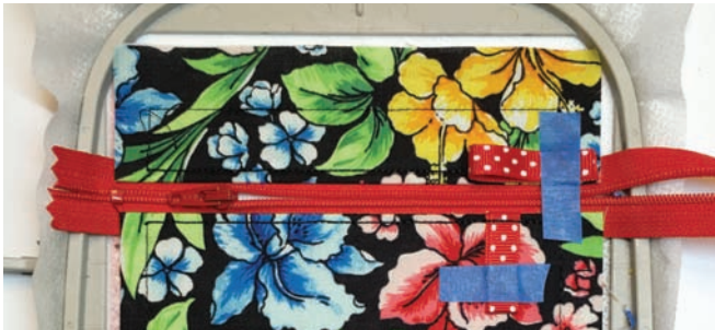
Figure 22. To add a loop, fold the loop in half, wrong sides together with the raw edges matching to extending into the seam allowance at least 1/4”.
