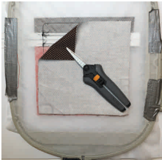
Figure 25. Place the back lining piece face down on the bottom side of the hoop. Tape diagonally across each of the 4 corners to secure for stitching.
