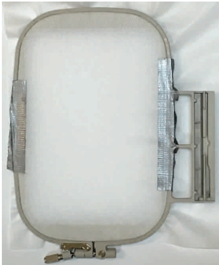
Figure 13. I like to use duct tape to prevent slippage.
