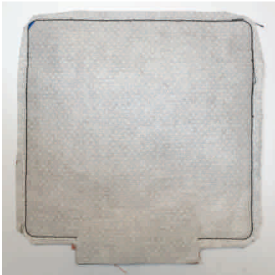
Figure 29. Trim seam allowances to about 1/4", trimming corners more closely. Leave an extension at the opening.
