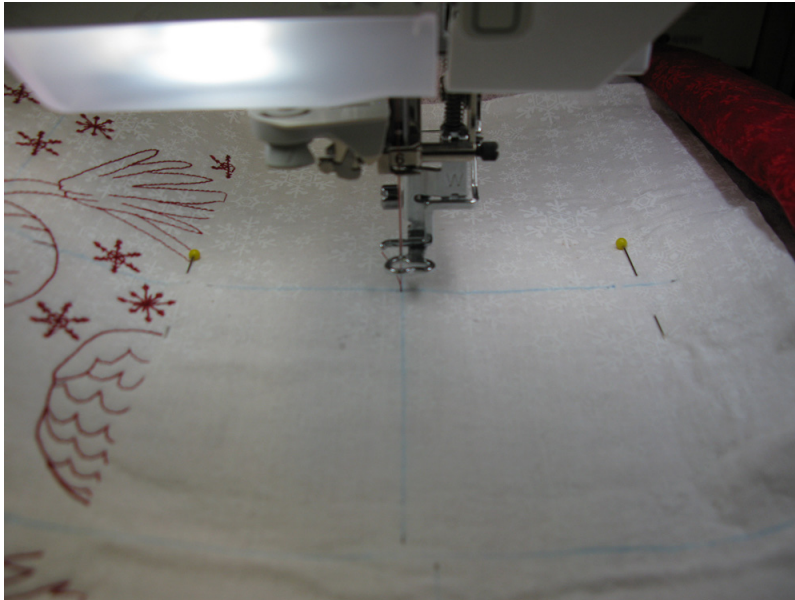
Figure 5. Start by centering the needle over the center of the marked design.
